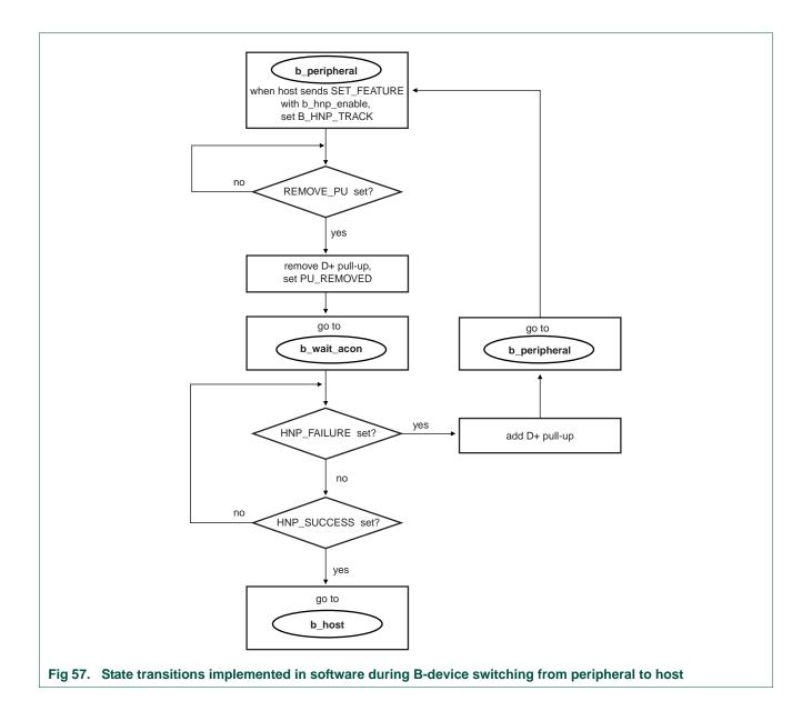
Note that only the subset of B-device HNP states and state transitions supported by hardware are shown. Software is responsible for implementing all of the HNP states.
