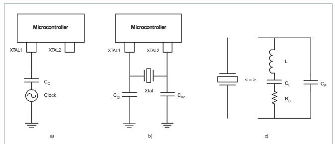
Fig 10. Oscillator modes and models: a) slave mode of operation, b) oscillation mode of operation, c) external crystal model used for  $C_{X1}/X_2$  evaluation
