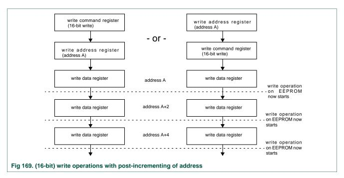
If the data register is written while a previous EEPROM operation is still pending, the write transfer on the system bus is stalled until the previous operation is finished. This can be avoided by polling the interrupt status register to see if an operation is still pending before starting the write operation.
