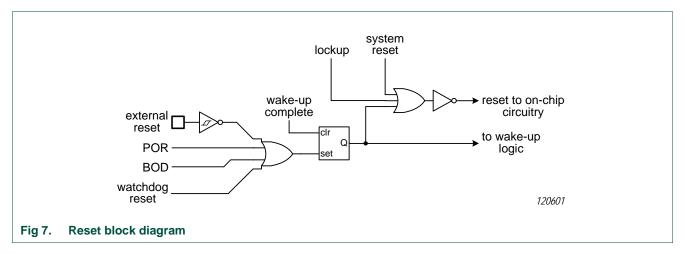
On the assertion of a reset source external to the CPU (POR, BOD reset, External reset, and Watchdog reset), the IRC starts up. After the IRC-start-up time (maximum of 60 µs on power-up) and after the IRC provides a stable clock output, the reset signal is latched and synchronized on the IRC clock. Then the following two sequences start simultaneously:
