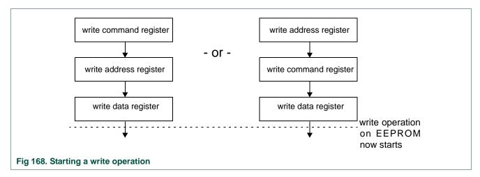
A write operation causes an automatic post-increment of the address. This allows consecutive writes to the page register without the need of writing a new address for every write operation. Of course the address register could be written with another address value to write to another location.
