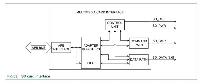
The SD card interface is a secure digital/multimedia memory card bus master that provides an interface to a multimedia card stack or to a secure digital memory card. It consists of five subunits:
