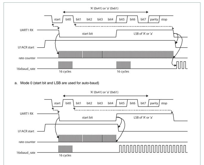
b. Mode 1 (only start bit is used for auto-baud)
