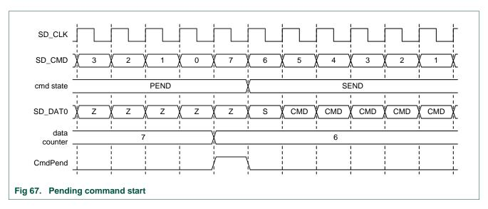
The data block counter determines the end of a data block. If the counter is zero, the end-of-data condition is TRUE (see <u>Section 16.7.9 "Data Control Register"</u> for more information).
