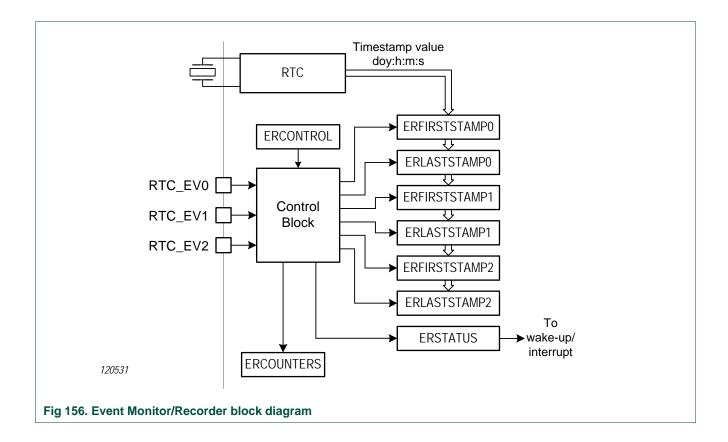
The CPU may at any time check the ERSTATUS register for events. If, for instance the EV0 bit is set, the corresponding ERFIRSTSTAMP0 and ERLASTSTAMP0 registers contain valid timestamps. The ERCOUNTER0 will also contain a valid count of the total number of events on channel 0 (up to a maximum of seven).
