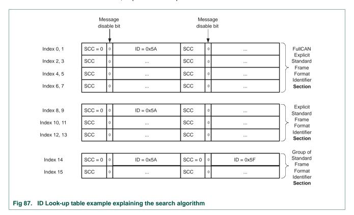
The identifier 0x5A of the CAN Controller 1 with the Source CAN Channel SCC = 0, is defined in all three sections. With this configuration incoming CAN messages on CAN Controller 1 with a 0x5A identifier will find a match in the FullCAN section.
