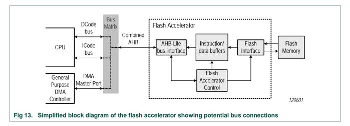
In the following descriptions, the term "fetch" applies to an explicit flash read request from the CPU. "Prefetch" is used to denote a flash read of instructions beyond the current processor fetch address.
