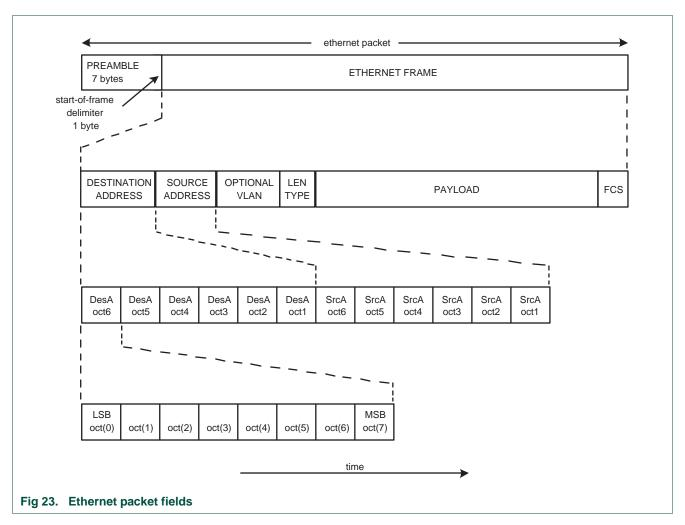
A packet consists of a preamble, a start-of-frame delimiter and an Ethernet frame.
