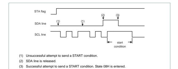
Fig 123. Recovering from a bus obstruction caused by a LOW level on SDA
