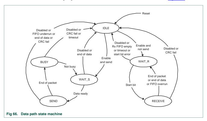
• IDLE: The data path is inactive, and the SD\_DAT[3:0] outputs are in HI-Z. When the data control register is written and the enable bit is set, the DPSM loads the data counter with a new value and, depending on the data direction bit, moves to either the WAIT\_S or WAIT\_R state.
