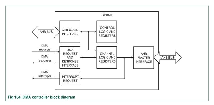
The functions of the DMA Controller are described in the following sections.
