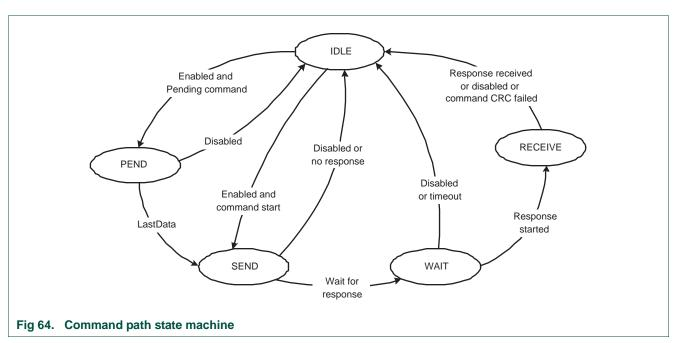
When the WAIT state is entered, the command timer starts running. If the timeout 1 is reached before the CPSM moves to the RECEIVE state, the timeout flag is set and the IDLE2 state is entered.
