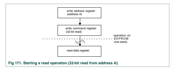
If the read data register is read while the read operation is still pending, then the read transfer on the system bus is stalled until the previous read operation is finished. This can be avoided by polling the interrupt status register to see if the operation is still pending before reading the read data register.
