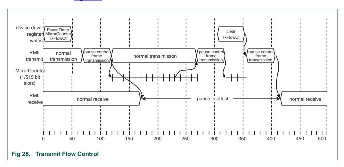
In this example, a frame is received while transmitting another frame (full duplex.) The device driver detects that some buffer might overrun and enables the transmit flow control by programming the PauseTimer and MirrorCounter fields of the FlowControlCounter register, after which it enables the transmit flow control by setting the TxFlowControl bit in the Command register.
