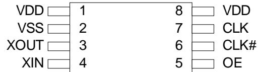
Figure 1. 8-pin TSSOP pinout
