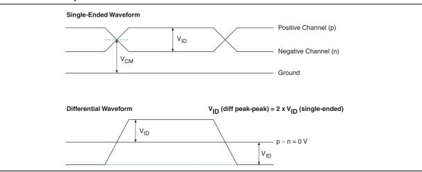
Figure 1–5 shows the transmitter output waveform.
