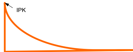
Figure 47. Input Charge Inrush Current
