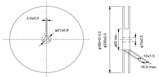
Fig.3 Taping Diagram
