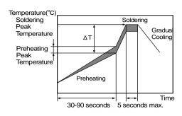
[Allowable Flow Soldering Temperature and Time]
