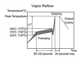
[Allowable Reflow Soldering Temperature and Time]
