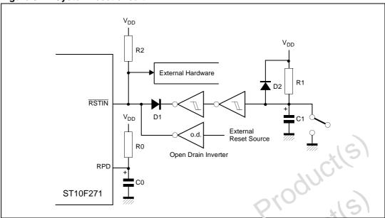
Figure 32. Internal (simplified) reset circuitry
