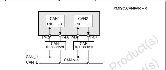
The ST10F271 also supports single CAN Bus multiple (Lal) interfaces using the open drain option of the CANx\_TxD output as shown in *Figure* (4. Thanks to the OR-Wired Connection, only one transceiver is required. In this case the design of the application must take in account the wire length and the noise or vironment.
