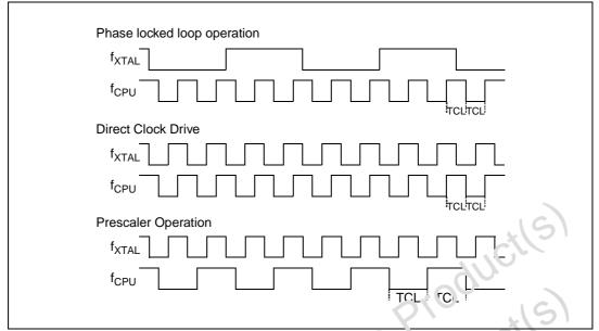
Generation mechanisms for the CPU clock
