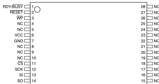
TSOP Top View Type 1
